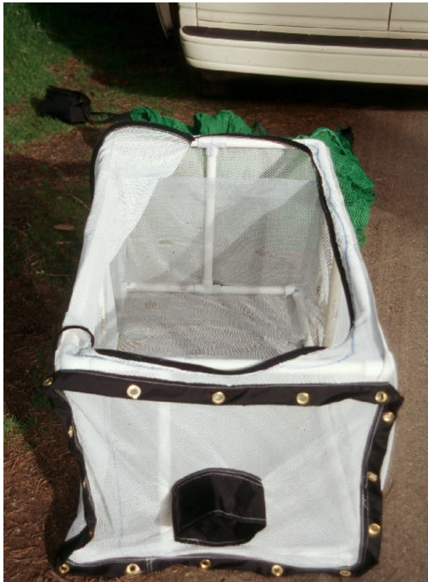
Figure 2: Live car box for outmigrant trap
